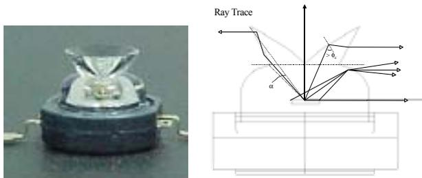
Figure 3: Luxeon™ Side Emitter with ray trace drawing
