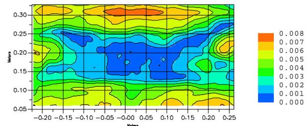
Figure 8: Measured Color uniformity  $\Delta u'v'$
