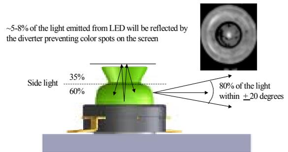
Figure 5: Optical Ray trace with diverter
