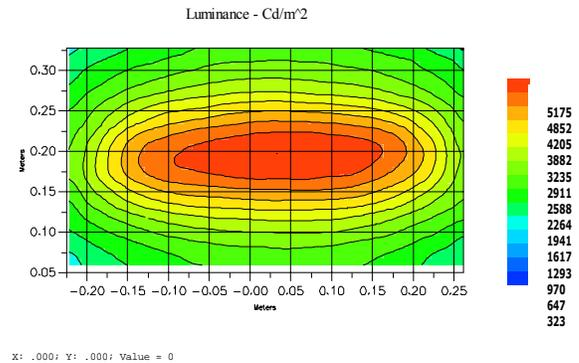
Figure 7: Measured Brightness uniformity
