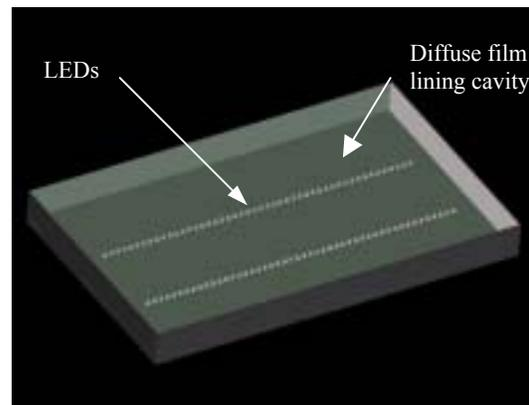
Figure 1: Typical RGB Layout within reflective cavity
