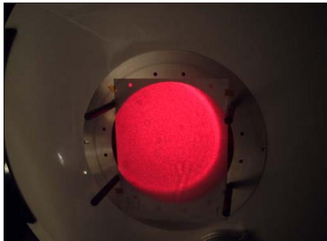
**Figure (5): Photograph of the beam incident on a Mylar sheet at the chamber exit.**
