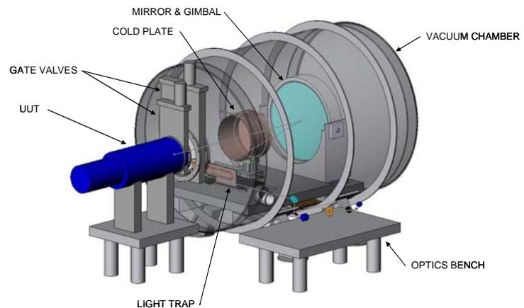
Figure (1): CAD model of the stray light test station.
