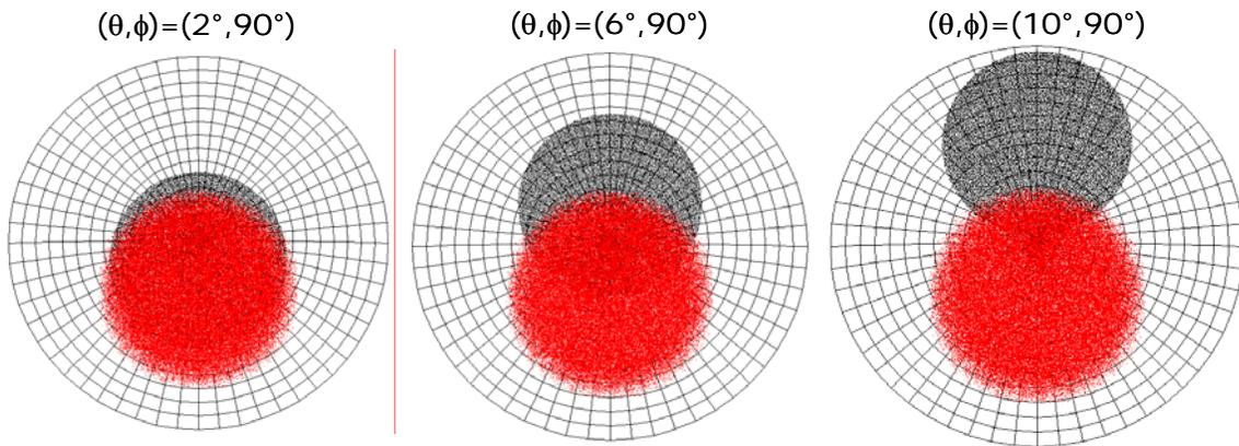
**Figure (8): Footprints of the beam (dark spots) and  $2^\circ \times 2^\circ$  sensor field of view (light/red spots) on the collimating mirror at three beam directions.**
