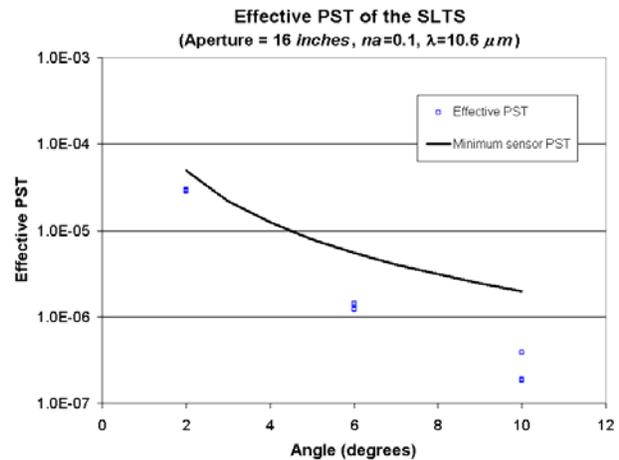
Figure (10): Effective PST (blue squares) and minimum sensor PST as a function of off-axis illumination angle (elevation) at a wavelength of  $10.6 \mu\text{m}$ .
