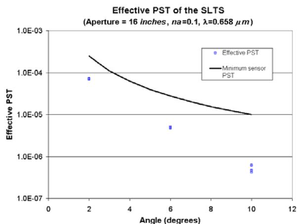
**Figure (9) Effective PST (blue squares) and minimum sensor PST as a function of off-axis illumination angle (elevation) at a wavelength of 0.658  $\mu m$ .**
