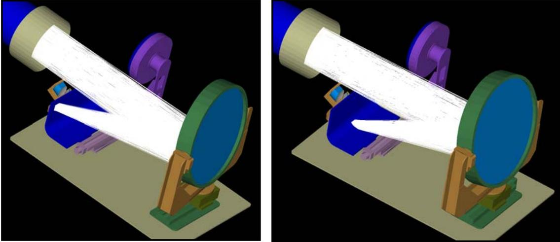
**Figure (3): Ray traces from the sensor show how the sensor’s field of view scans across the light trap as the collimating mirror shifts and rotates.**
