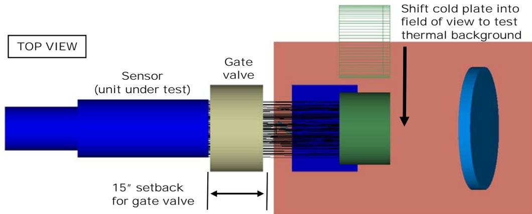
**Figure (4): Illustration of how a cold plate moves into the field of view of the sensor during a thermal background test.**
