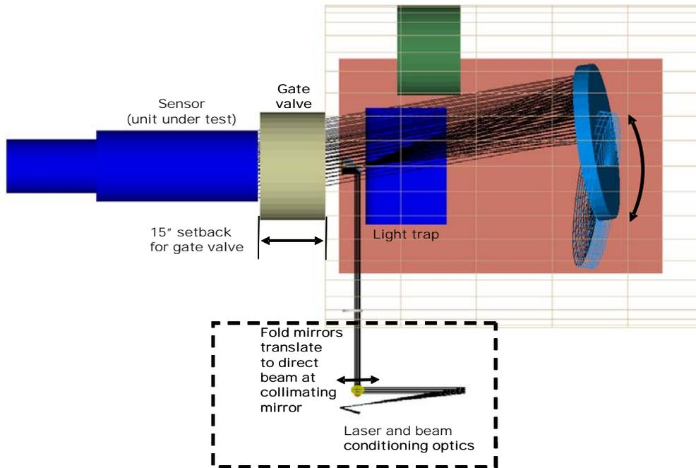
**Figure (2): Illustration of laser light propagating through the stray light test station.**
