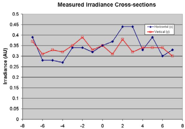
Figure (7): Beam irradiance as a function location on a vertical and horizontal cross section.
