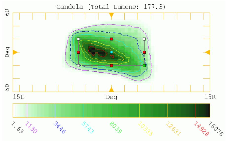
**Figure 1.12** Output view after creation of first segment
