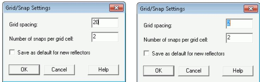
**Figure 1.9** Grid/Snap Settings for Reflector view (left) and for Output view (right)
