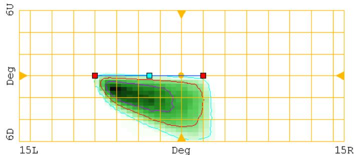
**Figure 2.8** Output pattern for segment S2 with filament used as source point
