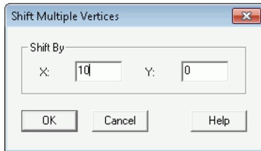
**Figure 2.15** Setting the shift for a group of vertices
