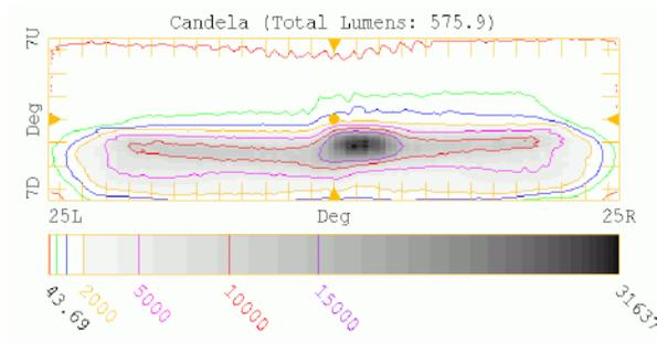
**Figure A.1** Output calculated by ReflectorCAD. Resolution is 70 pixels vertical and 100 pixels horizontal. Calculation quality is at the middle (default) setting. The standard ReflectorCAD source model for the 9005 bulb (with approximately 600 facets) was used.
