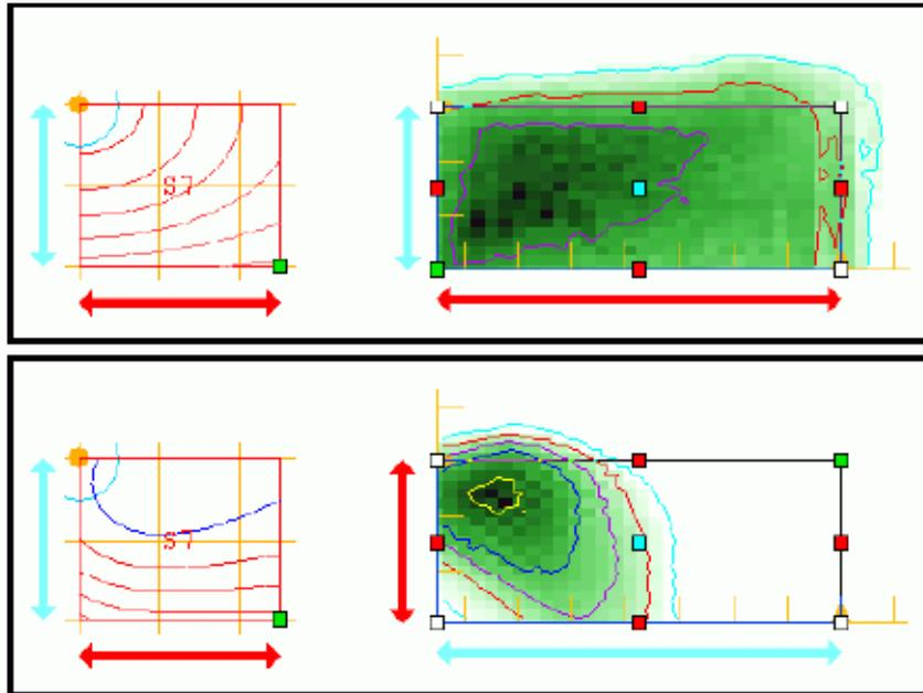
**Figure 2.13** The upper frame shows segment S7 aimed so that horizontal and vertical aim differences correspond to horizontal (red arrows) and vertical (cyan arrows) spatial differences, respectively. The lower frame shows the same segment with horizontal/vertical aim and spatial differences mismatched.
