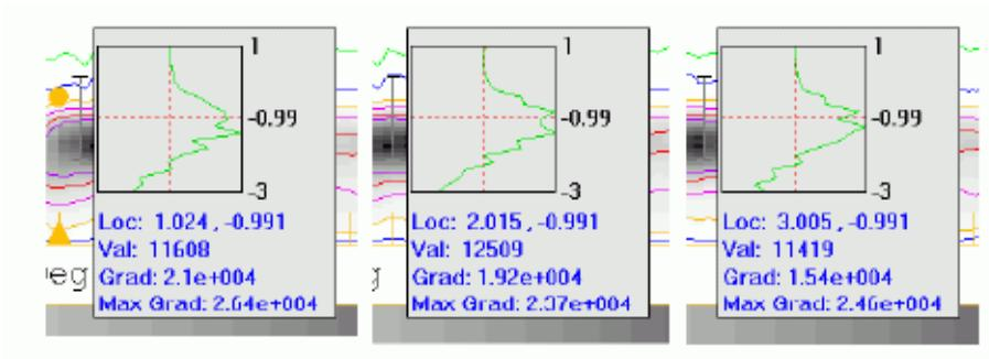
**Figure A.3** Vertical derivative for output slices along 1, 2 and 3 degrees right, as measured in ReflectoCAD, using the gradient query feature
