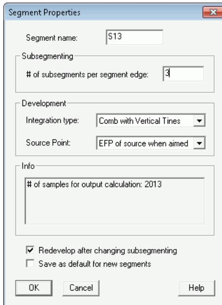
**Figure 2.11** Setting grid resolution (sub-segmenting)
