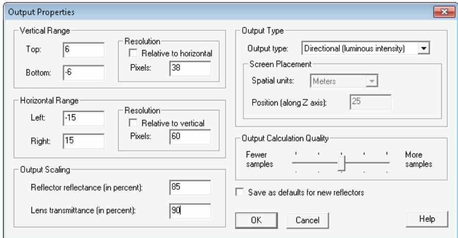
**Figure 1.8** Setting output properties
