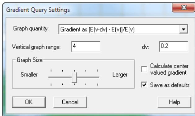
**Figure A.7** Gradient query settings used in ReflectorCAD for measurements shown in Figure A.6
