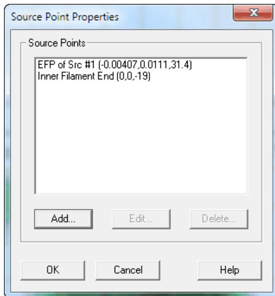
**Figure 2.6** Adding a source point at the inner filament end
