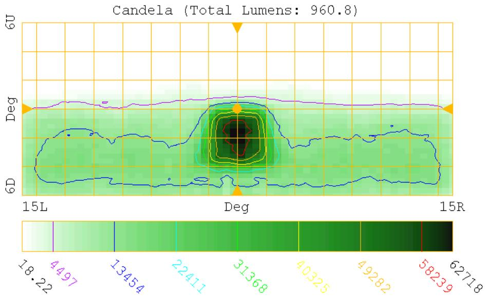
**Figure 1.30** Total output of finished reflector
