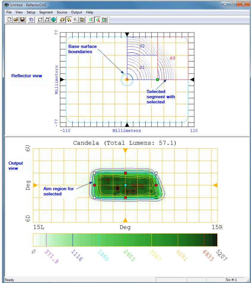
**Figure 1.1** ReflectorCAD window with key features delineated. (In this figure, the window is shown in its vertical layout, with the reflector view above the output view. The layout can be changed to a horizontal view on the **View** menu.)
