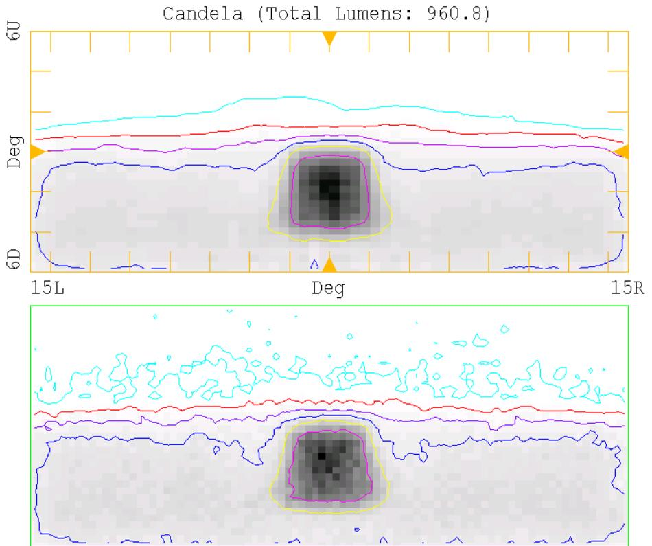
**Figure 2.3** Comparison of output calculated in ReflectorCAD (upper frame) and ASAP (lower frame). (The ASAP calculation used 500,000 source rays and yielded a total flux of 957 lumens. Contours were added manually in the ASAP display window.)
