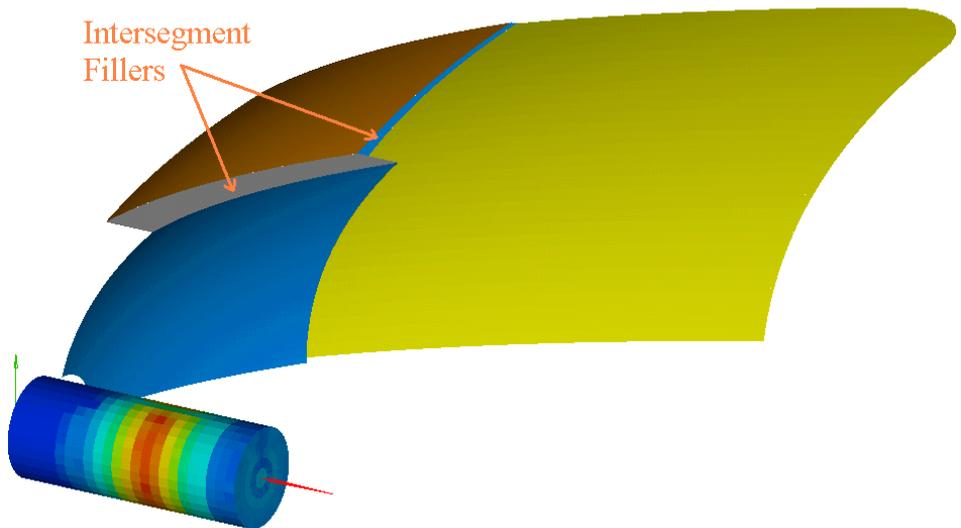
**Figure 1.23** 3D preview of reflector highlighting intersegment fillers
