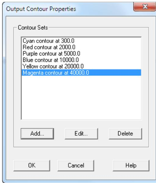
**Figure 2.1** Setting fixed contour levels
