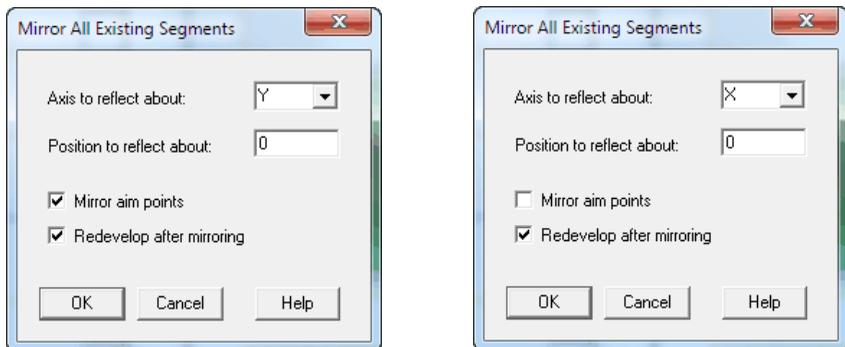
Figure 1.27 Mirroring about the Y axis (left) and X axis (right)
