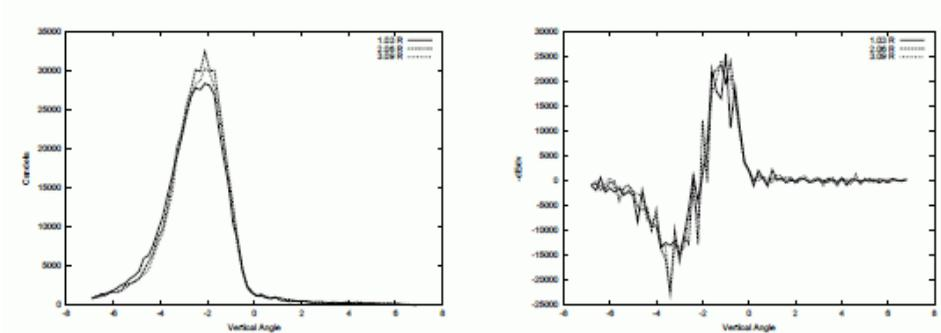
**Figure A.4** Vertical slices along 1, 2 and 3 degrees right, showing the output (left) and vertical partial derivative of the output (right), as calculated by ASAP
